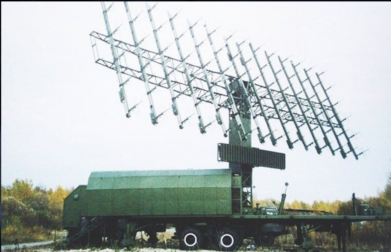
Transportable, 3D AESA VHF Radar 1L119 NEBO SVU (Rosoboronexport, Russia)
